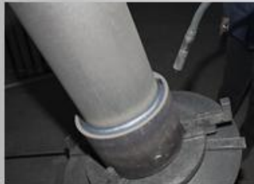
Large Diameter Steel Pipe Part Welding and Joint Test
